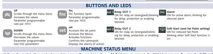
a) Press the 'set' button and release it to access the machine status menu. In normal conditions, the labels for the two Set point values are found in the menu. Once the 'SP1' label has been displayed, press the "set" button to display the Setpoint 1 value. The Setpoint 1 value appears on the display. To change the Set point
