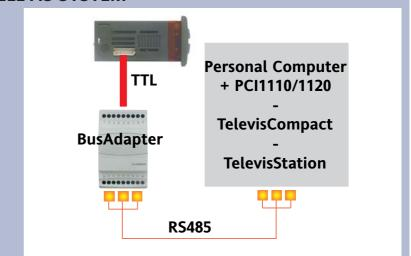
The Televis remote control systems can be connected using the TTL serial port (the 130 or 150 485 BUS ADAPTER TTL-RS interface module must be used). To configure the instrument to do this, you need to access the "Add" folder and use the "dEA" and "FAA" parameters.
