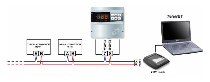
NET CONFIGURATION WITH MODBUS-RTU PROTOCOL
