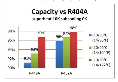
R452A delivers more capacity than R449A especially at low condensing temperatures.
