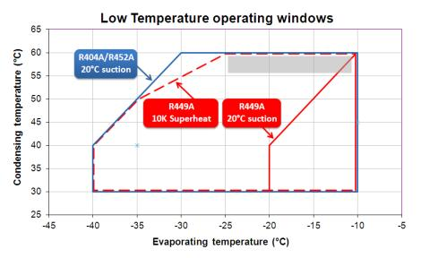
In cases where refrigerating systems using a reciprocating compressor would run at steady conditions into the shaded area of the above compressor application window, then Tecumseh advises to replace the current POE 32cst oil viscosity grade by a 68cst.
