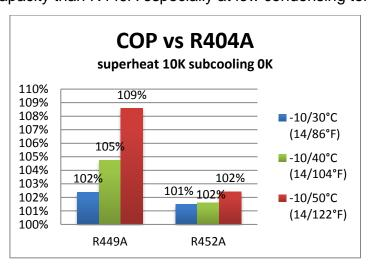
Refrigerants R449A and R452A both exhibit an efficiency gain over R404A, with a slight advantage for R449A. This is especially true at high evaporating and condensing temperatures.
