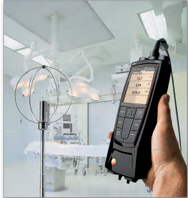
Turbulentiemeting in clean rooms
