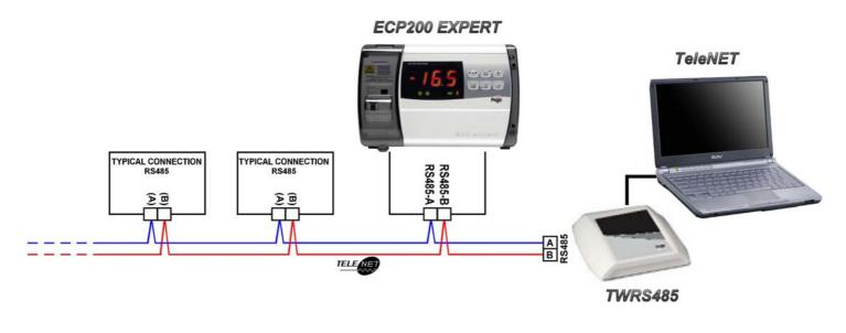
NET CONFIGURATION WITH MODBUS-RTU PROTOCOL
