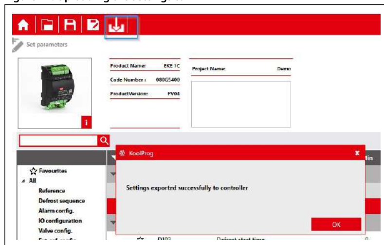
Figure 47: Uploading the settings to EKE
