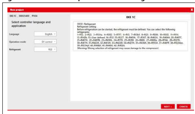
Figure 42: Wizard for Rapid Controller Configuration
