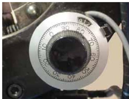
Electro Mechanical control with vernier dial
