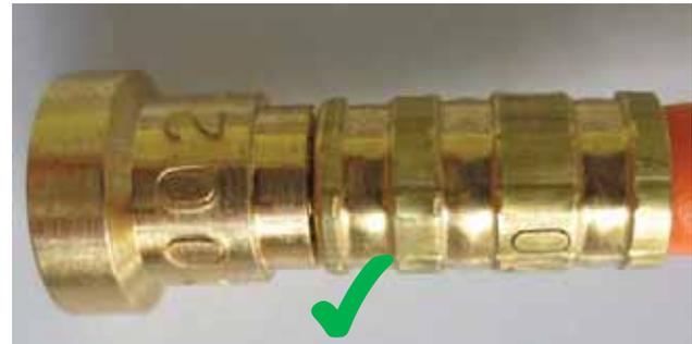
To have verification of correct crimping, carry out a check with a vernier.
