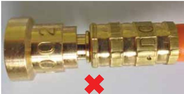
Insert not crimped in the proper position
