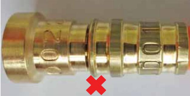
Example of ferrule not completely swaged
