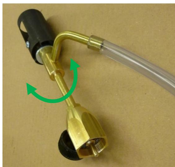
The arc must be installed loosely (movable)! If the arc is tightened the airflow could be cut off (→ yellow flame).
