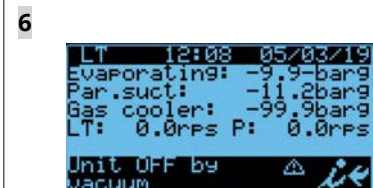
The status on the front screen will now indicate “Unit OFF by vacuum”, in this state the CDU cannot be set in ON. The above step should be reversed prior to charging the unit
