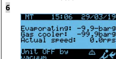
The status on the front screen will now indicate “Unit OFF by vacuum”, in this state the CDU cannot be set in ON. The above step should be reversed prior to charging the unit
