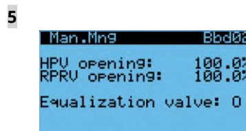
Set the wanted valves status during the Vacuum O = Open / C = Close
