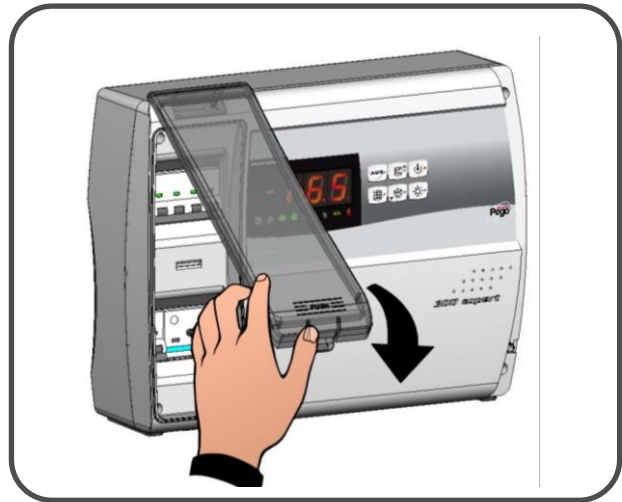
Fig. 4: Close the transparent protection cover.
