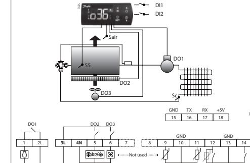
Note: 2L and 3L must be connected to the same phase.
