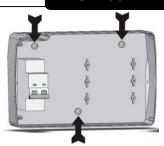
Fig. 7: Hook the front panel back on to the base of the box by re-inserting the hinges into their slots and making them bend. Rotate the panel downwards by 180° to access the PCB.
