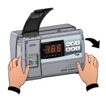
**Fig. 5:** Press on the sides of each hinge to unlodge it and completely remove the front panel.
